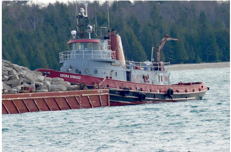
Tugboat Erika Kobasic hauls 1,300 - 1,400 tons of rock across Lake Michigan bound for Round Island Lighthouse in Lake Huron. Contractor is North Shore Marine Terminal Photo courtesy of Keepers of Round Island Lighthouse.
